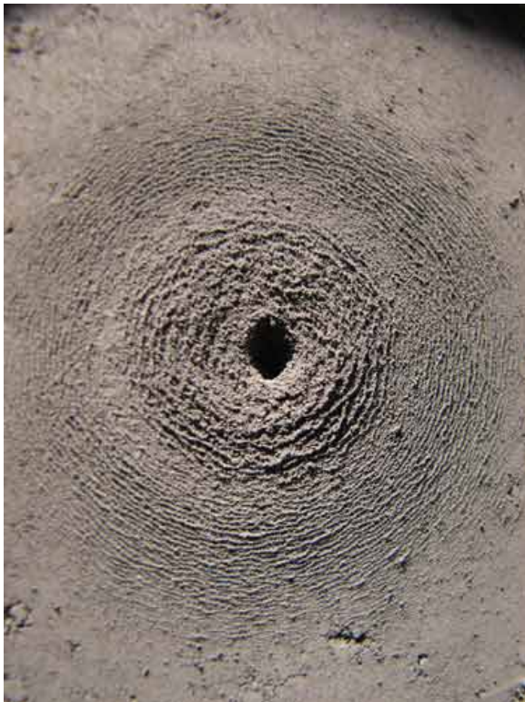
Figure 10. Laboratory result of an electric plasma discharge in air. Credit: Vemasat Labs
